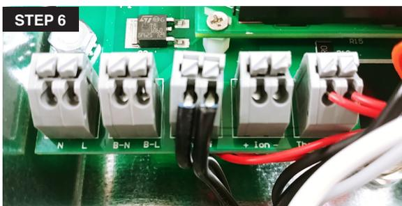
6. After the test is completed, unplug the unit and replace the wires in their original position. Black wire from the power cord connects into L and white wire from the cord connects into N. Black wire going to the ballast connects into B-L and white wire going to the ballast connects into B-N.
