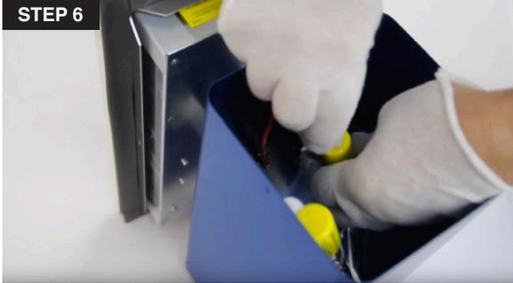
6. While holding the porcelain end-cap (with 4 pins) in the clamp, carefully push the white connector onto the four pins. The plug is designed so that it can only be installed one way. You may have to rotate the socket 90° to line up the pins with the holes. The connector will fit into position.
