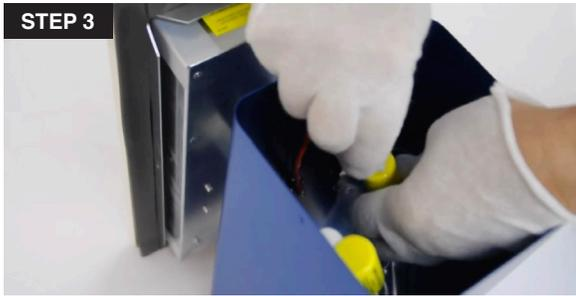
3. While holding the porcelain end-cap (with 4 pins) in the clamp, carefully push the white connector onto the four pins. The plug is designed so that it can only be installed one way. You may have to rotate the socket 90° to line up the pins with the holes. The connector will fit into position.
