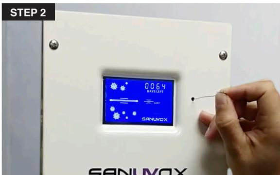
2. Use a small object similar to a paper clip and insert it into the hole in order to be able to press the reset button.
