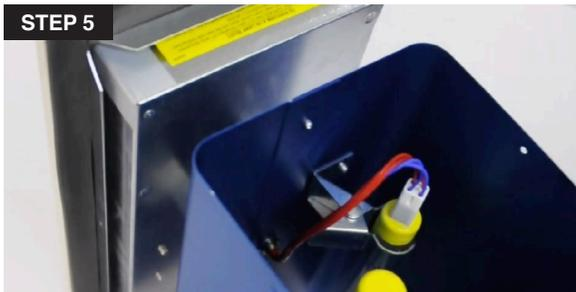
5. Once the UV lamp is inserted, release the clamp to fix the lamp in place.
