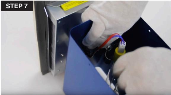
7. Slide the **UV lamp porcelain end-cap (with 4 pins)** in the aluminum tube of the unit, then through the clamp.
