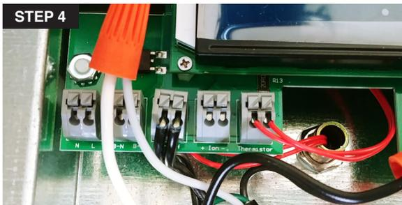
4. Disconnect N and B-N and join them together using twist-on wire connectors
