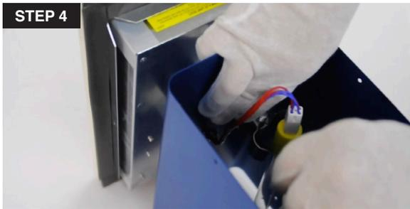
4. Slide the **UV lamp porcelain end-cap (with 4 pins)** in the aluminum tube of the unit, then through the clamp.
