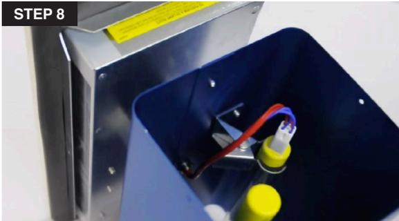
8. Once the UV lamp is inserted, release the clamp to fix the lamp in place.
