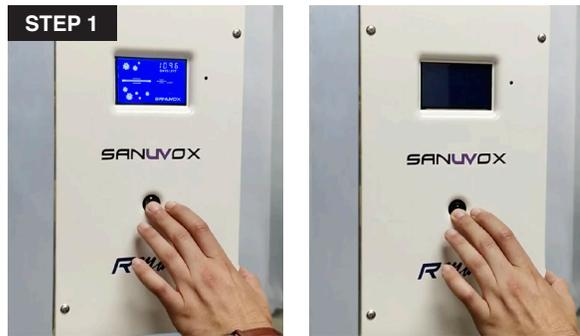
1. If your unit is powered ON, start by turning OFF the power switch.
