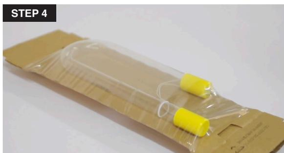
4. **Prepare the new lamp.** Remove the contents from packaging. Only after you have visually inspected the UV lamp should you break the security seal on the underside of the cardboard sleeve.
