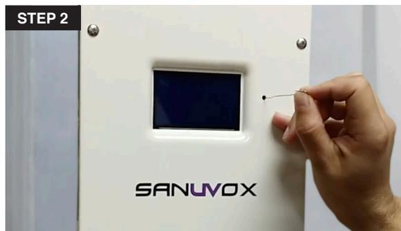
2. Use a small object similar to a paper clip and insert it into the reset hole in order to be able to press the reset button.
