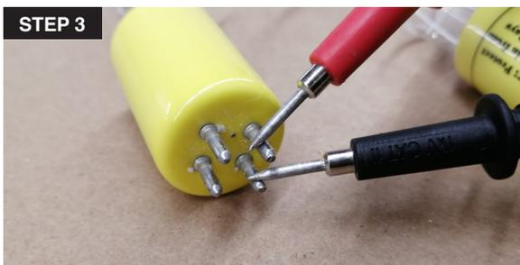
3. Using an ohmmeter place 1 probe on 1 of the 4 pins and by sensing the 3 remaining pins, one should have continuity. Make sure the 2 remaining pins also have continuity. When both sets of pins test good for continuity, it can be assumed that the lamp is good.
