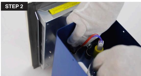
2. Remove the UV lamp from the lamp socket by opening the retaining clamp and pulling the UV lamp out of the reflector chamber.
