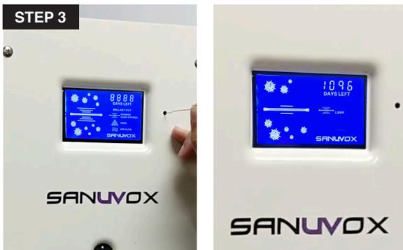
3. Press and hold the reset button for a minimum of 3 seconds. When releasing the reset button, the counter will be reset and the "Days Left" on the LCD screen will reset to 1096 days.
