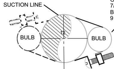
ON 7/8" AND LARGER LINES, MOUNT SENSING BULB AT EITHER THE 4 OR 8 O'CLOCK POSITION. NEVER MOUNT THE SENSING BULB ON BOTTOM OF LINE.
