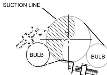
**NOTE** — NEVER MOUNT SENSING BULB ON BOTTOM OF LINE.
