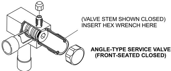
When service valve is **CLOSED**, the service port is open to the line set and indoor unit.
